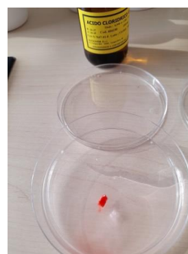
Fig. 19: Normal gelatine hard cps type 4 in HCL 0,1 N bath : after 15 minutes full dissolved.
