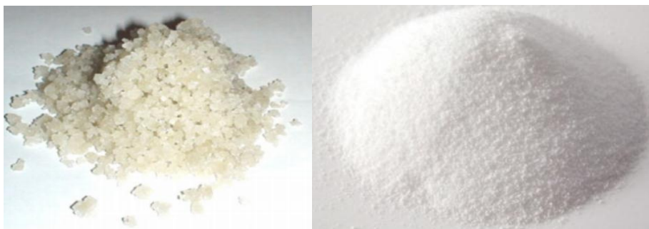
Figure-4: Salt from brine from its yellowish/off white color is bleached by chemical process-stripped of its minerals like Calcium, Magnesium by bleaching with chemical process.
