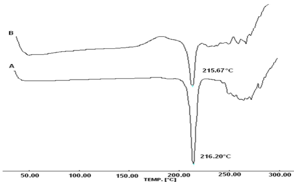
Figure 2: Differential Scanning Colorimetry of A) Pure drug Paracetamol and B) Drug with *A. auriculiformis* mucilage.
