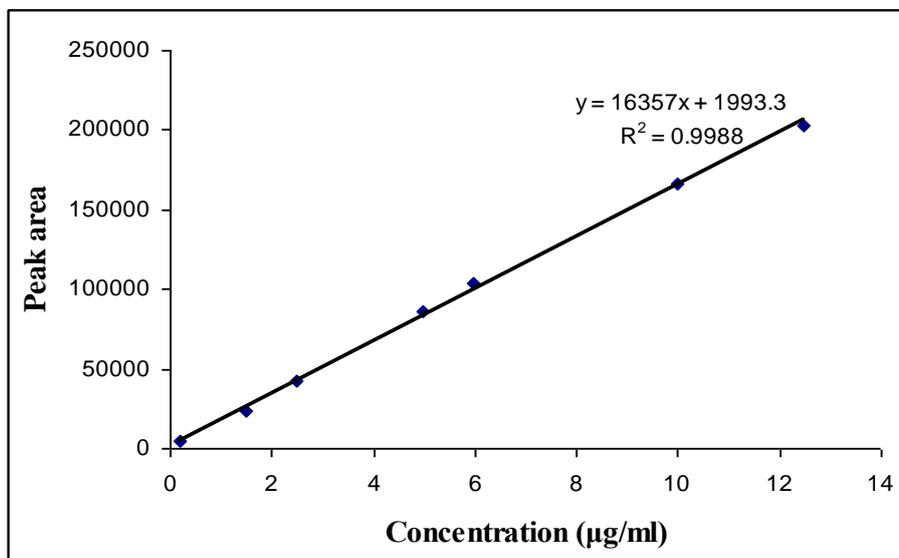
**Fig 10: Linearity plot for impurity C.**
