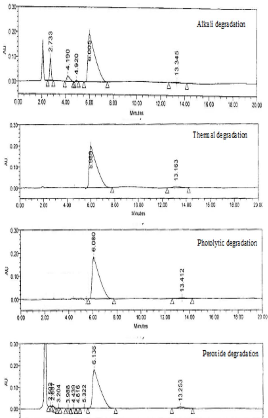
**Fig 6: Forced degradation chromatograms for Clopidogrel bisulphate.**
