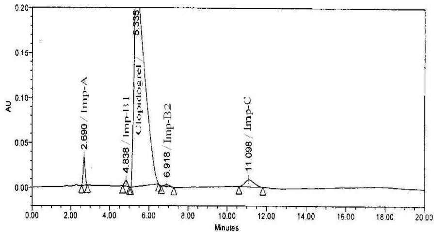
Fig 5: Typical chromatogram for Clopidogrel bisulphate spiked with impurities.
