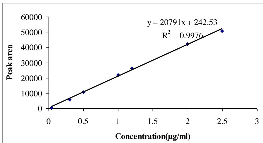
**Fig 7: Linearity plot for impurity A.**
