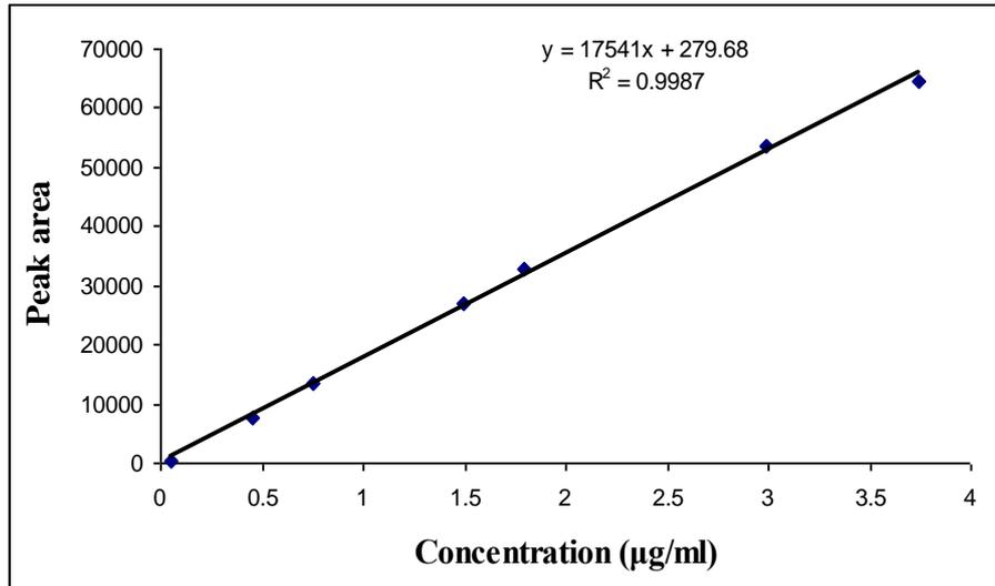
**Fig 9: Linearity plot for impurity B2 (Second Enantiomer)**
